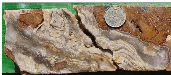
Colloform banding of silica at the Makedontsi deposit, typical of low sulphidation epithermal gold system
