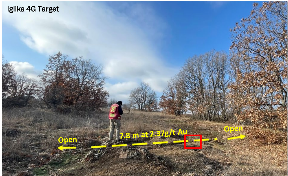
Surface channel sampling at 4G Target returns 7.8m grading 2.37 g/t gold, including 1.0m grading 12.3 g/t gold.
