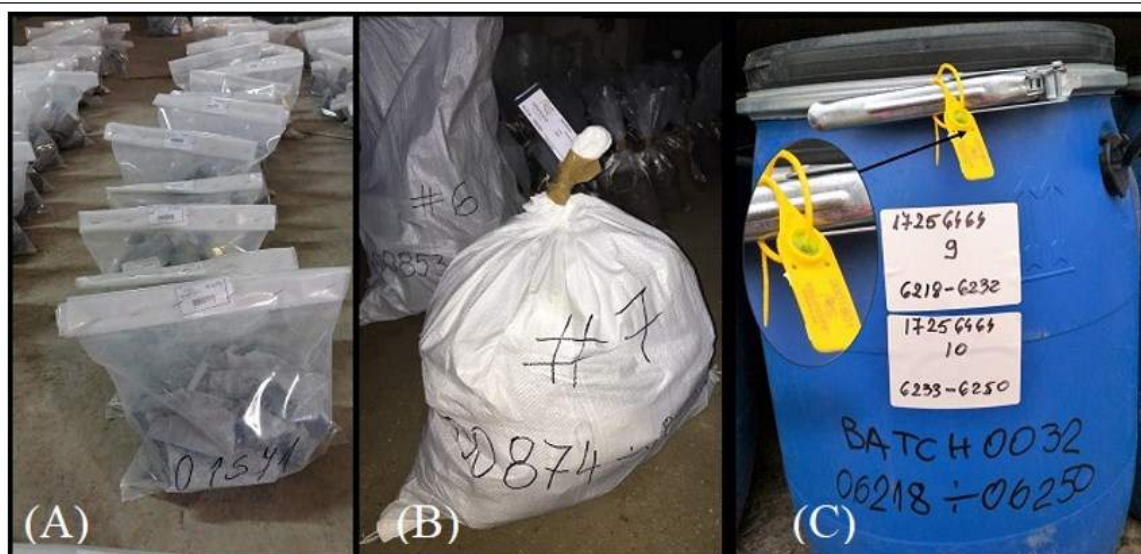
(A) Individual sample bags with sample tags (B) Polywoven bag labelled with sample sequence, (C) Plastic drum with sample and batch sequence and plastic tag seal
