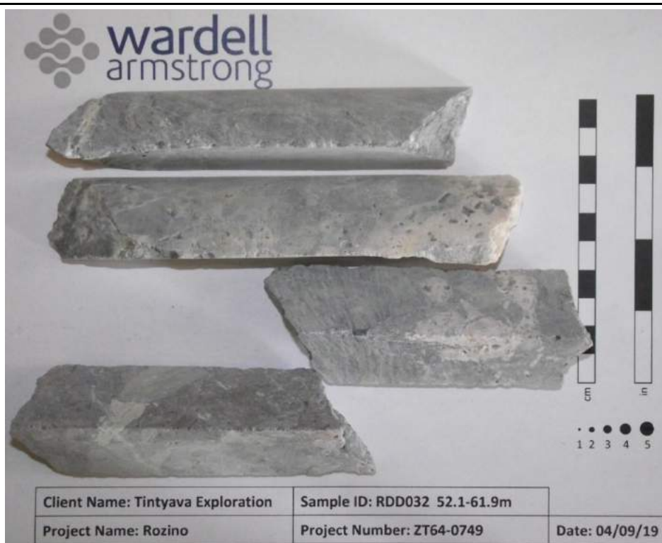
Figure 13-8 : Vein Zone Composite, RDD032 52.1-61.9 m interval (Source: WAI, 2019)
