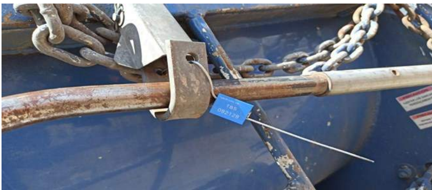
Figure 17-8 : Example of concentrate truck security tagging and sealing
