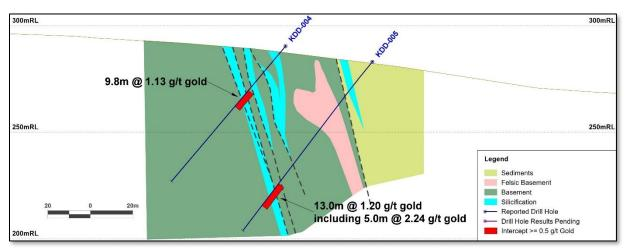
Figure 2: Drill section showing significant intersections at the Kazak East target. Drill results are pending for additional drill holes and drilling is ongoing.
