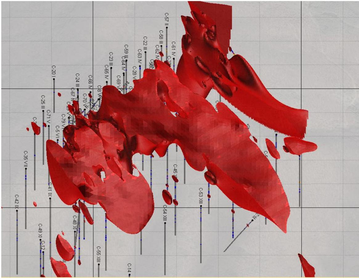
Figure 25.3: 3d view of Main Rozino deposit area and 0.5 g/t Au Implicit grade shells looking North (grid square 100m).
