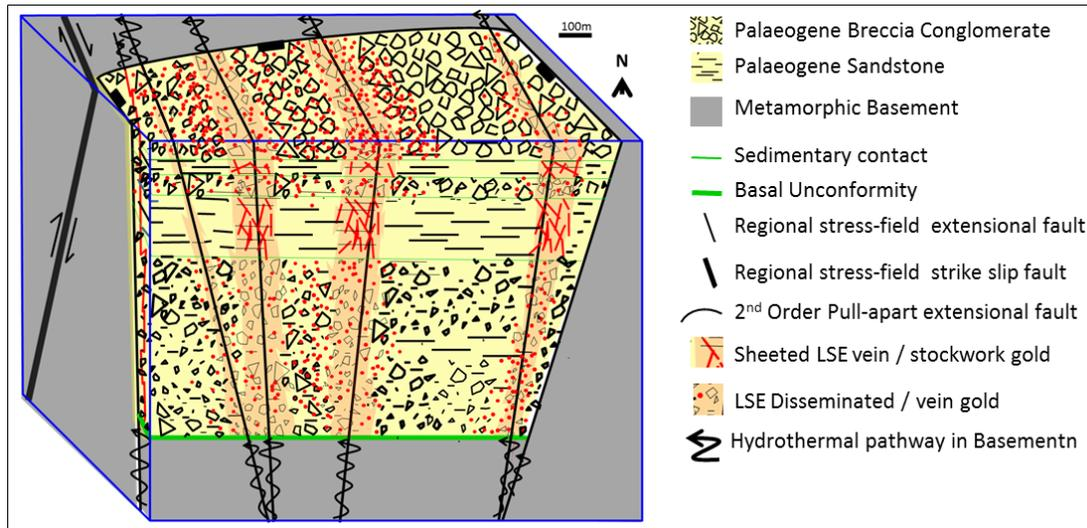
Figure 8.2: Schematic model for the Rozino Project sediment hosted LSE Deposit, Bulgaria
