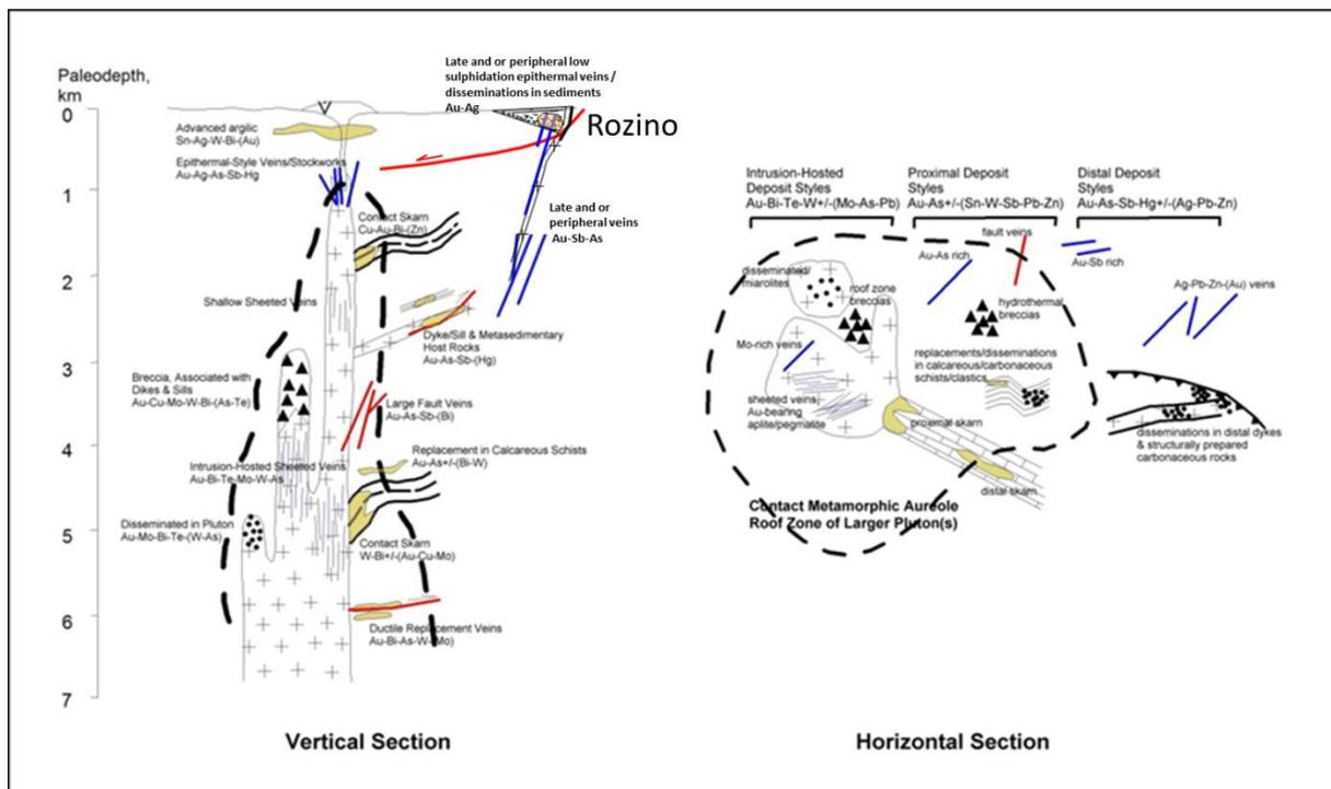
Figure 8.1: Schematic geological-exploration model for a reducing Intrusive-Related Gold Systems (IRGS) (modified from Lang, 2001)
