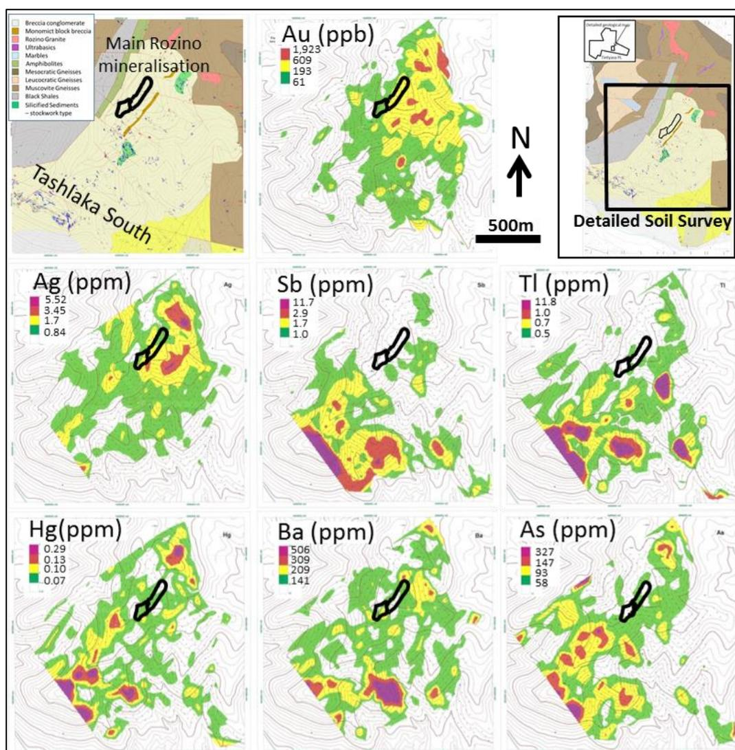
Figure 9.2: Soil anomaly maps for the detailed sampling programme at the Rozino Project (Andrew C, 2009). “Main Rozino mineralisation” outline represents a historic grade shell at basal contact and northeast arm of economic mineralisation above basal contact (projected to surface).
