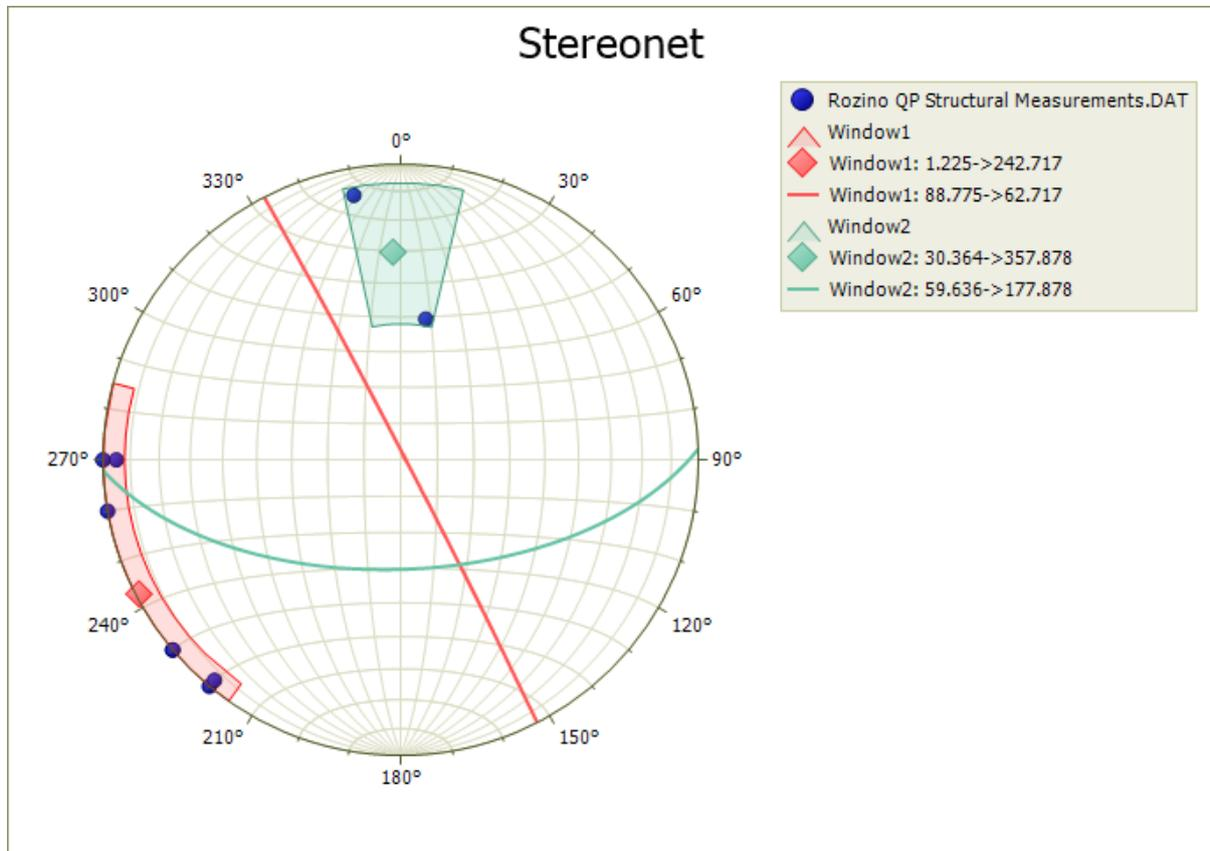
Figure 12.5: Stereonet of structural reading.
