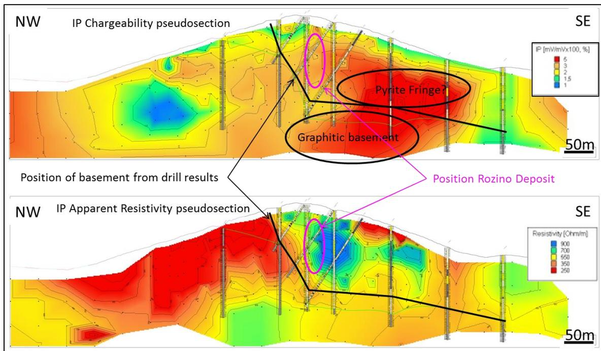
Figure 9.5: Chargeability and Apparent Resistivity pseudosections of Profile 7N oriented NW-SE across the Rozino Project (Andrew C, 2009)
