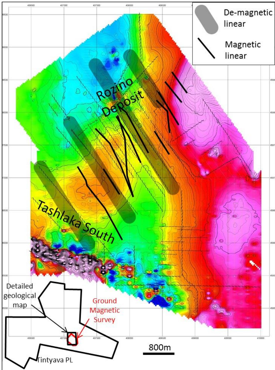
Figure 9.4: Compiled magnetic interpretation superimposed on Total Magnetic Intensity image of ground magnetic data collected at the Rozino Project (Andrew C, 2009)
