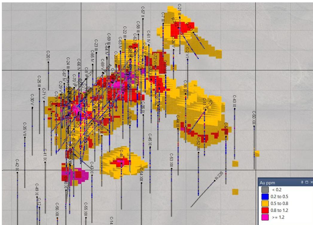
Figure 25.2: 3d view of Main Rozino deposit area and Hereward block model looking North (grid square 100m).
