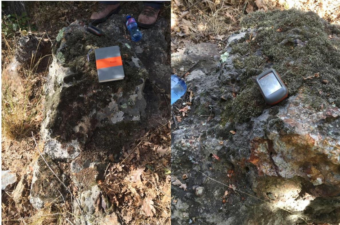
*Figure 12.2: Location 8a: NW trending silicified conglomerate with Fe-Cb veining (Sample AMSR01)*
