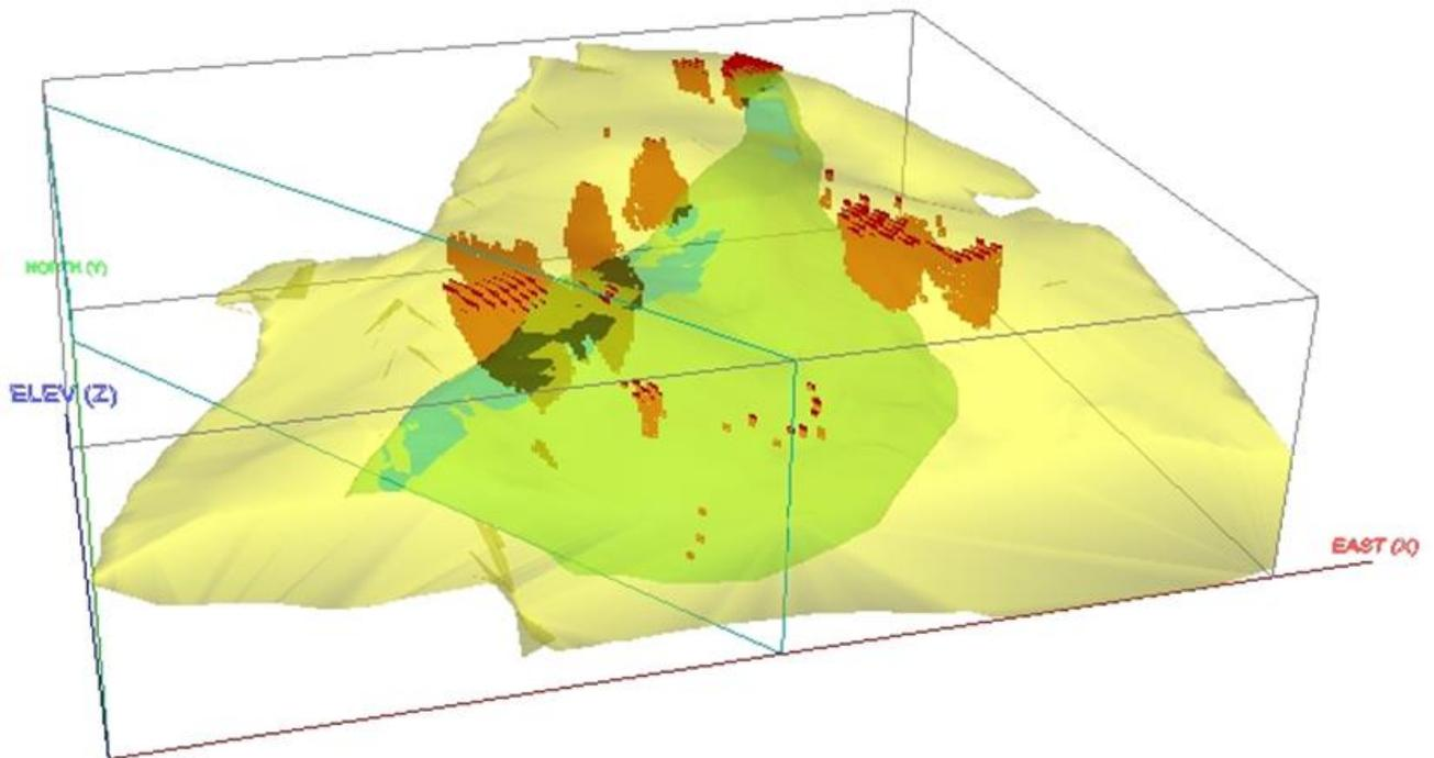
Figure 14.1: Three dimensional view of the Rozino block model using a 1.2 g/t Au cut-off grade. Initial search ellipsoid secondary axis range (40m) is less than the drill fence separation (50m). The contact between the Palaeogene and basement is shown as a green plane.
