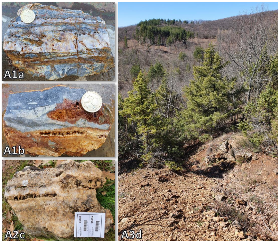
Plate 1: Photographs of rocks located within the new soil anomalies. A1a Amethyst vein breccia (0.26 g/t gold) and A1b comb quartz veining and silicified hydrothermal breccia (3.62 g/t gold). A2c epithermal cocks comb quartz vein (0.84g/t gold). A3d Photo viewing SW of shallow dipping low sulphidation epithermal vein in metamorphic basement (28.62 g/t gold).
